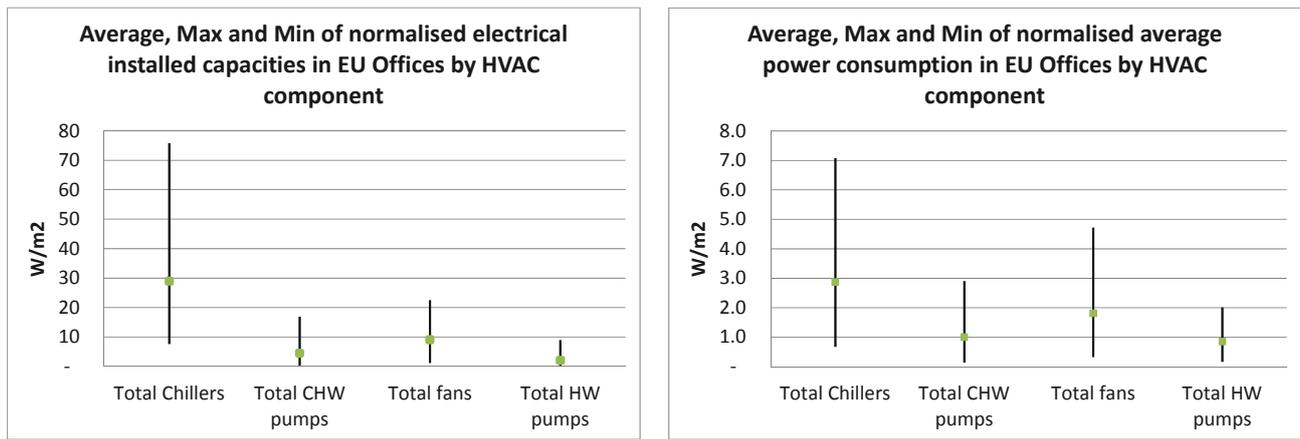
**Figure 3.** Average, Maximum and Minimum Installed and Annual Average Measured Power Demands normalized for floor area for Chillers, Chilled Water Pumps, Air Handling Units and Hot Water Pumps installed in EU Offices.
