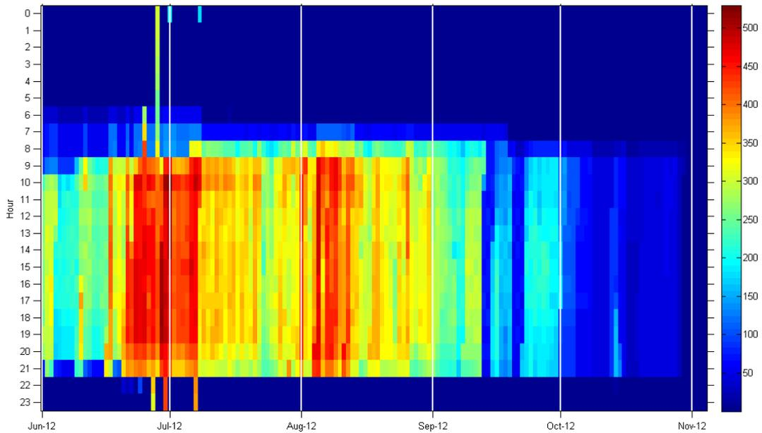
**Figure 2: Rooftop electric consumption of building A (kWh)**
