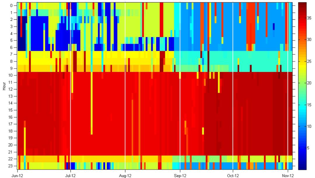
**Figure 3: Lighting electric consumption of building G (kWh)**
